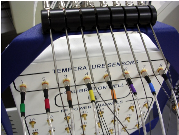
Figure 3-7: Microwave and Thermometry Interface Panel with sensors connected
