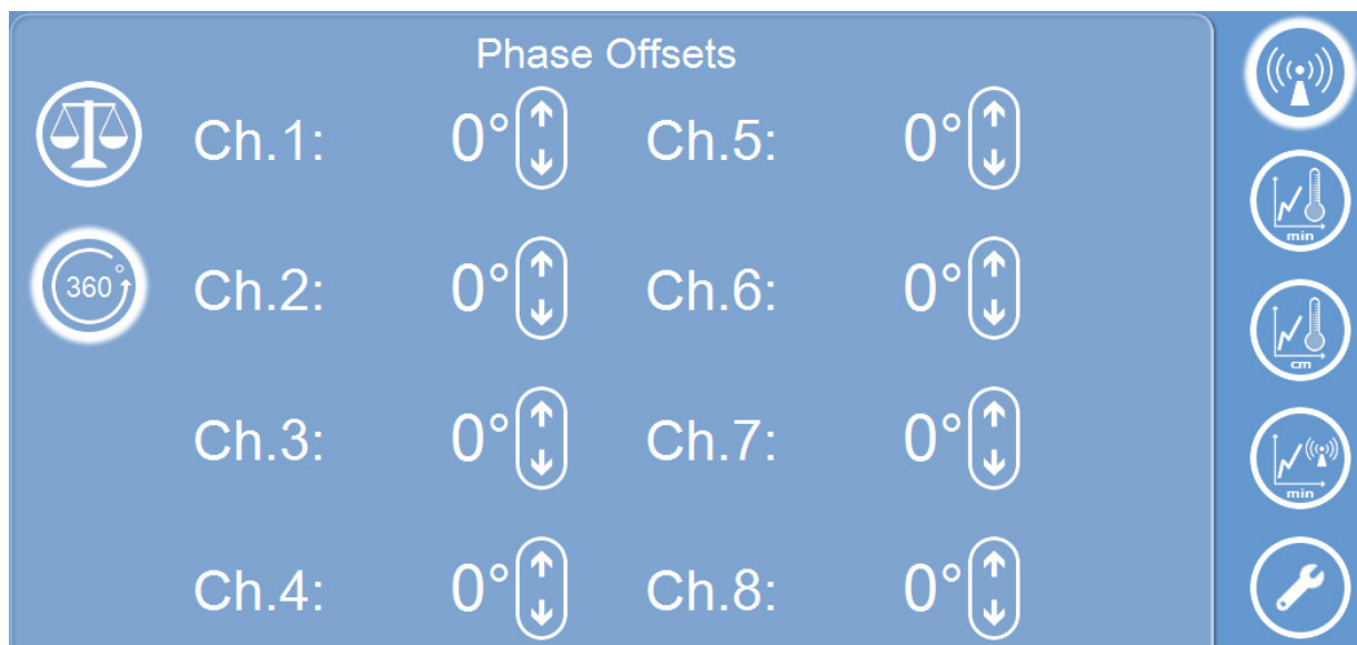
Figure 4-41: Phase Offsets Control Screen (Multiple Channel Applicator) – Synchronous Mode Only
