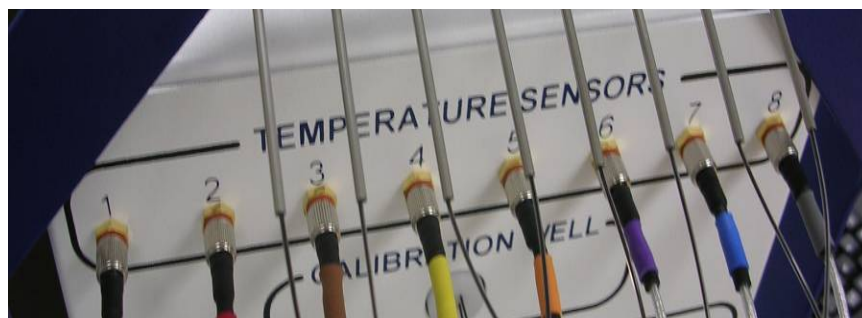
Figure 4-3: Temperature Sensor connection to Microwave and Thermometry Interface Panel
